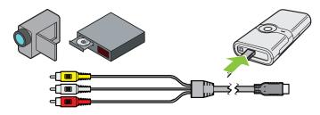
Tip: Some video devices do not have the standard audio and video connections and may require an AV cable specified by the manufacturer. The AV cable allows you to connect your video device to your TV monitor or your projector and may be purchased from the video device manufacturer. Once you have the AV cable, you may need the cable adapters to connect the video device cable and the projector cable.
